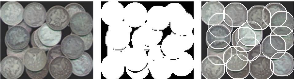
Fig. 5. Application of the proposed approach to an image containing overlapping coins. Although not all objects are detected our approach reveals promising results and recognizes even highly occluded models. Left: input image. Center: local pre-segmentation obtained by inspecting the distance to the background color and local thresholding; used as input to the proposed method. Right: segmented result.
