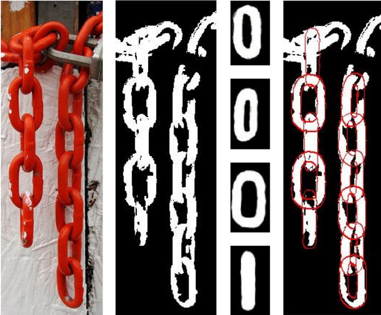
Fig. 6. Application of the proposed template-based segmentation approach to a real-world image. Left to right: original image, local pre-segmentation using a thresholded distance to the color red as foreground indicator, shape templates used for segmentation, and the final result. Note that even highly overlapping parts are labeled correctly.
