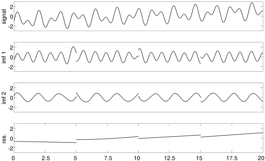
Fig. 2. EMD decomposition of a toy signal. The time series has been segmented into four segments and decomposed with EMD. After joining the resulting IMFs together, boundary effects become clearly visible at  $t = 5$ ,  $t = 10$  and  $t = 15$ .
