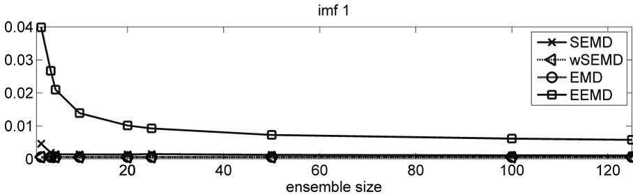
Fig. 6. Evolution of the mean of the absolute values of  $m(t)$  for SIMF/IMF 1 obtained with SEMD, weighted SEMD, EMD, and EEMD of the toy data with respect to the ensemble size is depicted.
