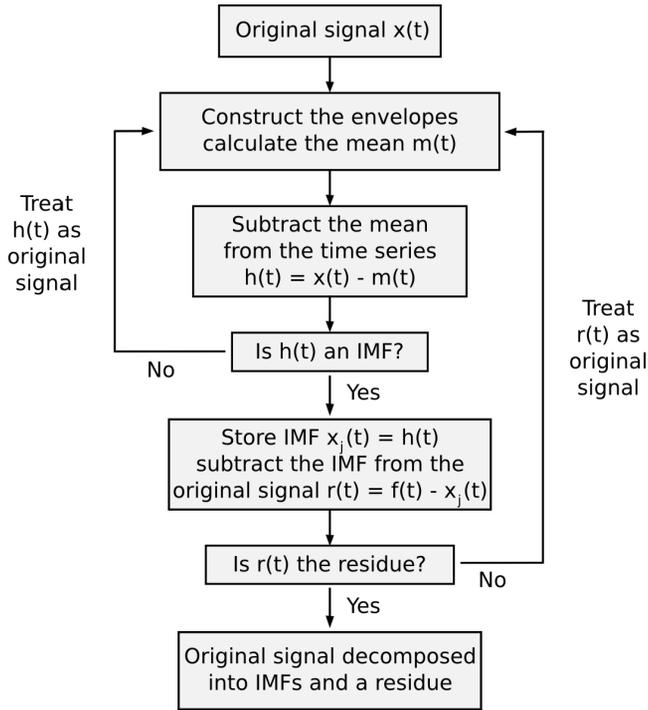
Fig. 1. Flowchart describing the principle mode of operation of EMD.
