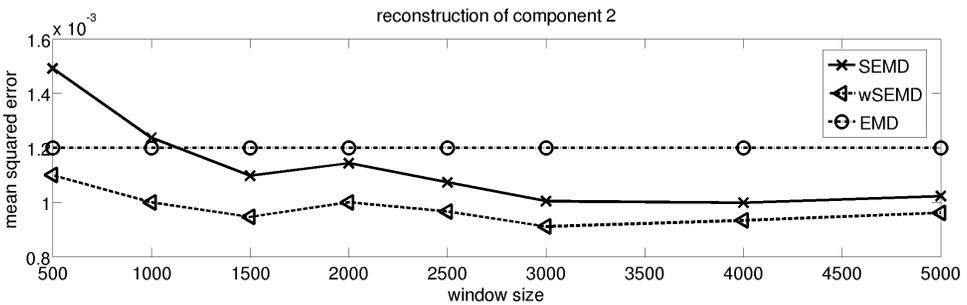
Fig. 14. Reconstruction error for component 2 of the toy data after the decomposition with SEMD, wSEMD, and EMD as a function of window size.
