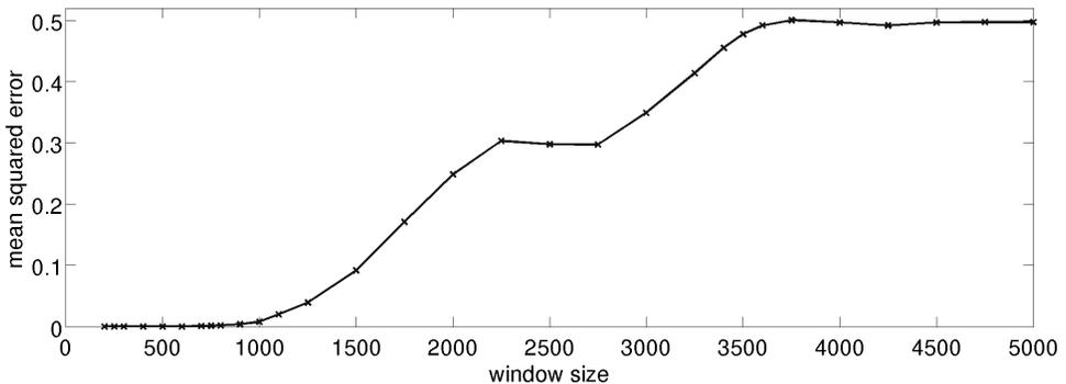
Fig. 12. MSE of the sliding residuum compared to the sinusoidal toy data as a function of the window size. The number of estimates was  $E = 50$ .
