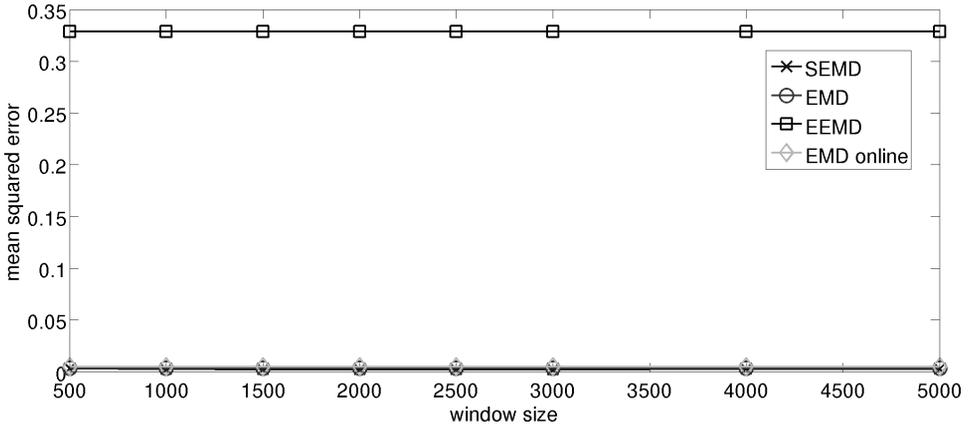
Fig. 17. Summed up reconstruction error of all components obtained with SEMD, EMD, EEMD, and on-line EMD as a function of window size.
