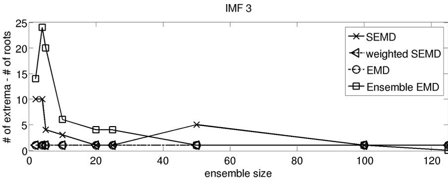
Fig. 9. Evolution of the difference between the number of extrema and zero crossings of IMF 3 obtained with SEMD, wSEMD, EMD, and EEMD of the toy data with respect to the ensemble size.
