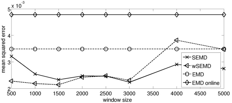
Fig. 18. Summed up reconstruction error of all components obtained with wSEMD, SEMD, EMD, and on-line EMD as a function of window size.
