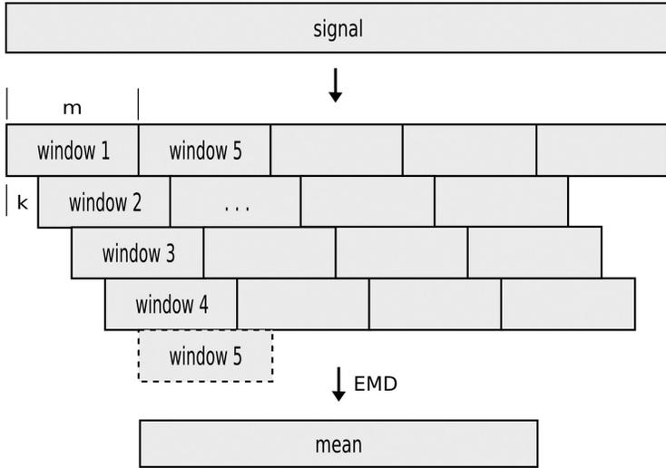
Fig. 3. Schema of the SEMD algorithm. The time series segments in the shifted windows are EEMD. IMFs and the residuum are determined finally by mode amplitudes which are averaged over corresponding samples in all windows.  $m$  describes the window size and  $k$  the step size.
