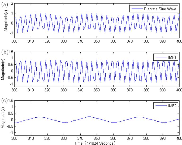
Fig. 2. Sine wave and IMF(s): (a) Sampling signal of sine wave, (b) Decomposition results  $IMF_1$  and (c) pseudo-mode component  $IMF_2$  (simulation condition: sampling frequency is 1,024 Hz and signal frequency is 330 Hz).
