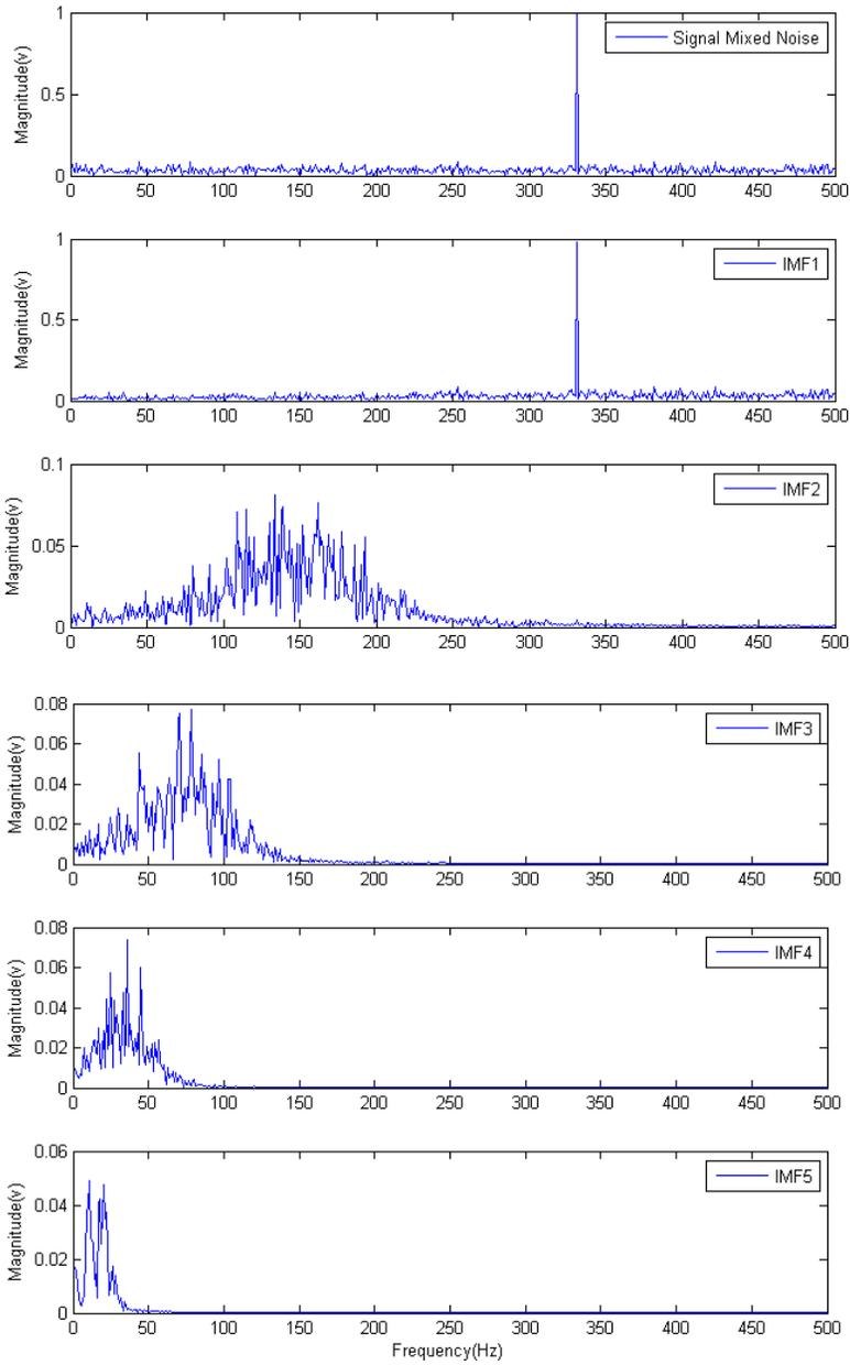
Fig. 6. EMD decomposition on a sine wave mixed with white noise — no mode error: and pseudo-mode harmonics caused by insufficient sampling rate (the ratio of white noise to sine wave of 0.6, sine wave with frequency 330 Hz and sampling frequency of 1,024 Hz).
