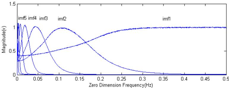
Fig. 4. Filter bank frequency domain characteristic of EMD decomposition.
