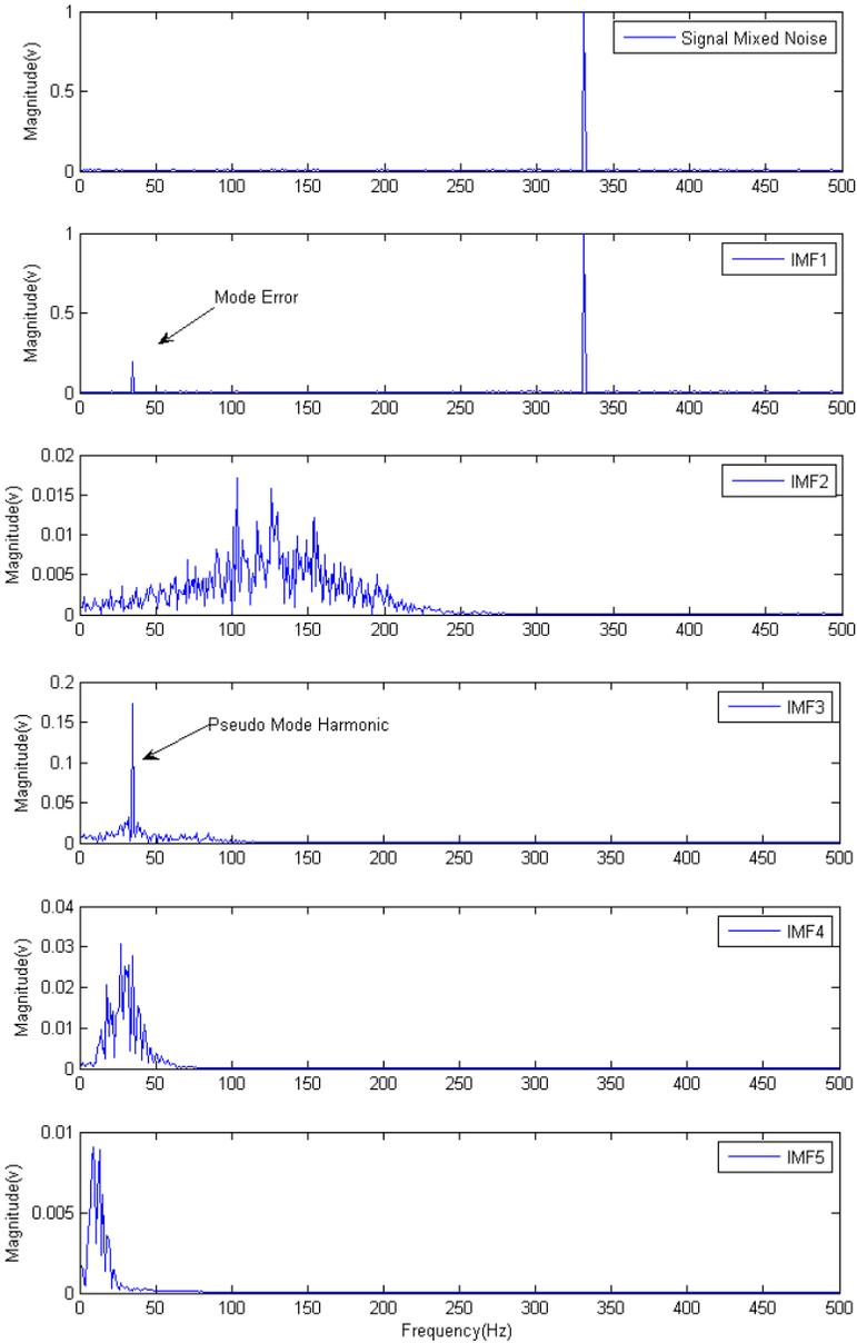
Fig. 5. EMD decomposition on a sine wave mixed with white noise: (a) (the ratio of white noise to sine wave of 0.1, sine wave with frequency 330 Hz, and sampling frequency of 1,024 Hz).
