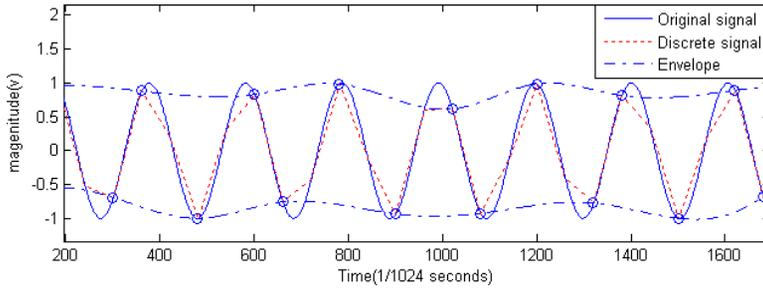
Fig. 1. Sketch of deviation in envelope computation caused by insufficient sampling rate.
