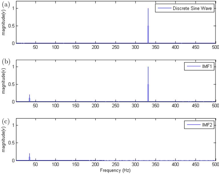
Fig. 3. Spectrum of sine wave and IMF(s): (a) Sampling signal of sine wave, (b) decomposition result IMF<sub>1</sub> and (c) pseudo-mode component IMF<sub>2</sub>.
