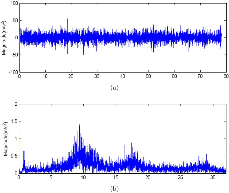
Fig. 7. Vibration acceleration and its spectrum: (a) Bearing vibration acceleration signal and (b) spectrum of bearing vibration acceleration.
