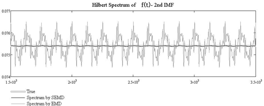
Fig. 8. The Hilbert spectrum of second IMF decomposed by SEMD and EMD in test signal  $f(t)$ .
