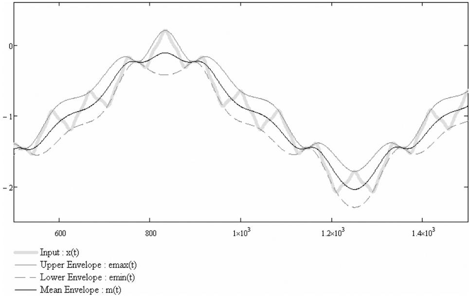
Fig. 1. Construct the envelopes by Cubic Spline passing through all extrema of Input  $x(t)$ . These envelopes can be replaced by other functions, for example, piecewise straight lines.
