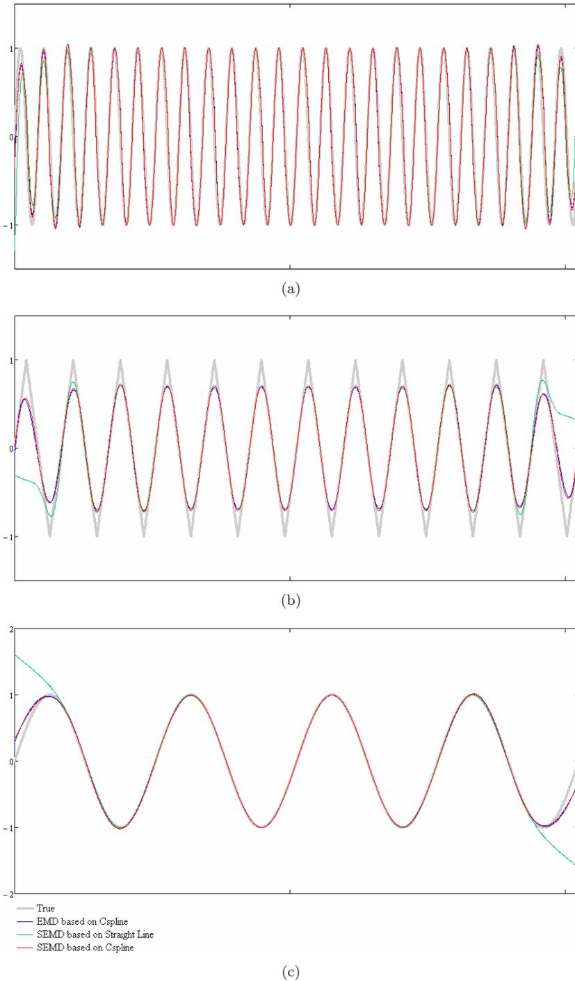
Fig. 11. Comparison between EMD and SEMD based on Cubic spline and straight line (a) The 1st sinusoidal component at 24 Hz (b) The 2nd saw teeth component at 12 Hz (c) The 3rd sinusoidal component at 4 Hz.
