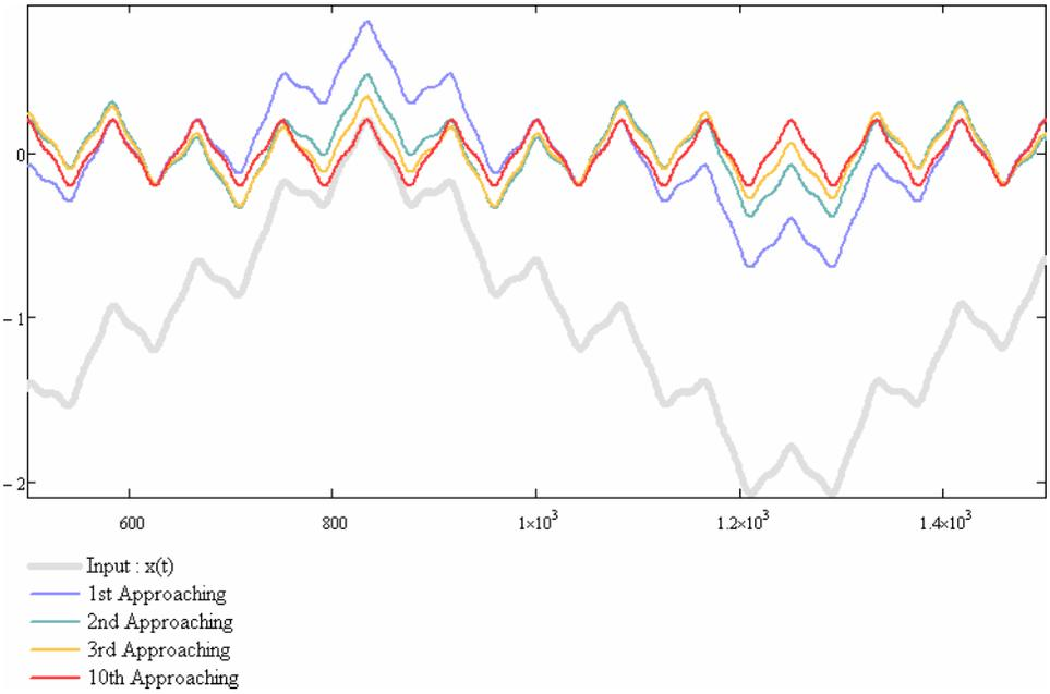
Fig. 3. The Smoothing-Sifting is the procedure to remove the smoothed mean from original data  $x(t)$  recursively.
