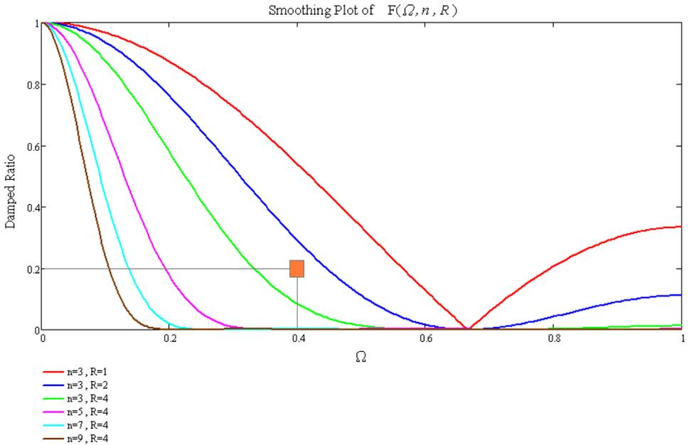
Fig. 5. For example: Trust only 20% (**Damped Ratio = 0.2**) of smoothed mean at digital frequency  $\Omega = 1.257$ , therefore, the curve  $n = 3$  and  $R = 4$  is conservatively chosen (Green line).
