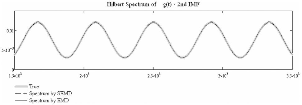
Fig. 9. The Hilbert spectrum of second IMF decomposed by SEMD and EMD in test signal  $g(t)$ .
