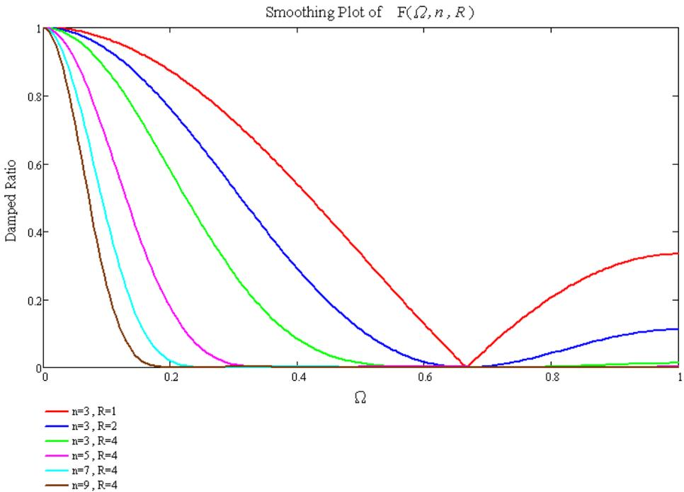
Fig. 4. The correlation between digital frequency  $\Omega$  and damped ratio  $R$  at a given window  $n$  and  $R$  times smoothing.
