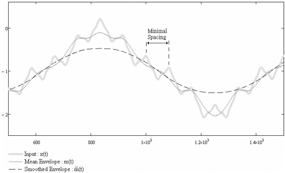
Fig. 2. Smoothed envelope is come from the moving average of mean  $m(t)$  with a given window. The smoothing window is altered adaptively by minimal spacing which is the least distance between extremes of  $x(t)$ .
